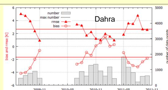
The land cover at Dahra, Senegal, is tiger bush with a TCC of 4%. The long data gap from Dec 2009 to Jun 2010 is due to theft of solar panels. Due to its sub-tropical climate, Dahra has the fewest data points of the four stations (many cloudy satellite pixels).
