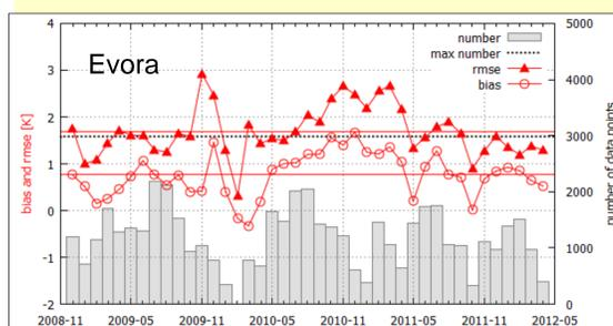
Radiometers observe grass and the crown of an oak tree near Evora, Portugal. A tree crown cover (TCC) of 33% determined for August 2009 gives the best correlation between satellite and in-situ LST. This agrees with the mean TCC of 29% determined by Carreiras et al. (2006).
